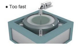
The photoresist splatters off of the substrate.
