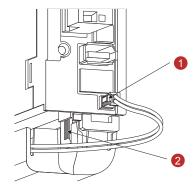
3 Slide in a new battery before inserting the plug into CN4.
