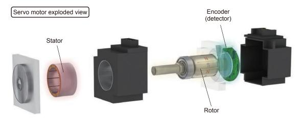
A servo motor is made up mainly of three parts: stator, rotor, and encoder.
